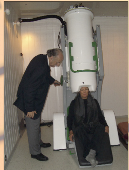
Biophysicist Photios Anninos, PhD (Laboratory of Medical Physics, University Hospital, Democritus University of Thrace, Greece) prepares for Superconductive Quantum Interference Device (SQUID) for testing.
